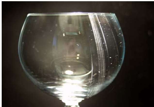
Image 3: Line corrosion (source: Proceedings of the 77 th Glass Technology Conference in Leipzig in 2003, pp. 55-58)
